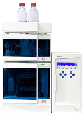
Figure 8: Recommended instrument configuration for this application: the ALEXYS Disulfides Analyzer, Au. The system consists of a P6.1L pump with integrated degasser, an AS6.1L autosampler, and the DECADE Elite electrochemical detector with Dual Cell Control (DCC).
